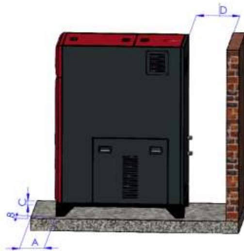
A: At least 80 cm is required for comfortable use of the cleaning arm and technical service actions;
