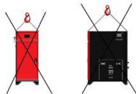
Due to the heavy weight of the product, special care should be taken during handling to the installation place. The net weight of each product is already indicated in the technical specifications table. Therefore, the equipment that has sufficient capacity for the lift action should be used during handling.
