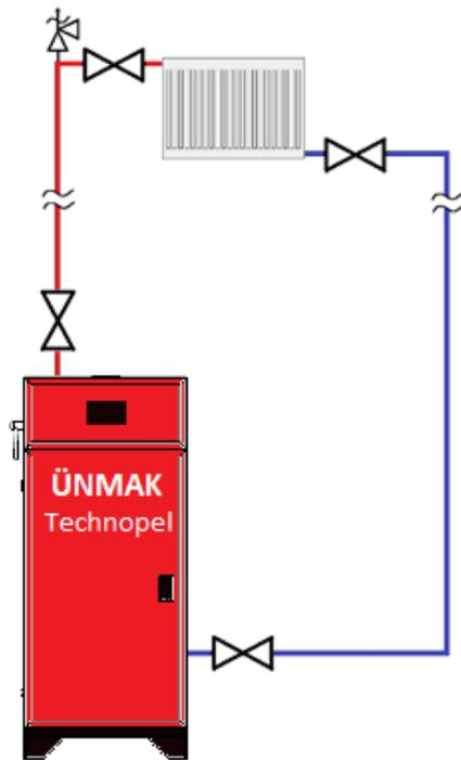
The equipment such as circulation pump, expansion tank, the safety valve is included with the pellet boiler, and no need to add on to the installation when the hydronic connection of the boiler is completed. It can be easily installed as the wiring diagram shows.
