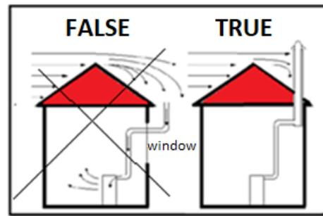
Wrongly installed flue and correctly installed flue and flue cap
