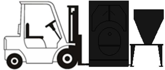
In order not to damage the boiler outer sheets and the boiler during transportation; While carrying the boiler with the help of a crane or hoist by passing a carrying rope through the forklift stands on its chassis, care should be taken that the carrying rope does not damage the painted thin sheets of the boiler and the reducer-fan group under the bunker.
