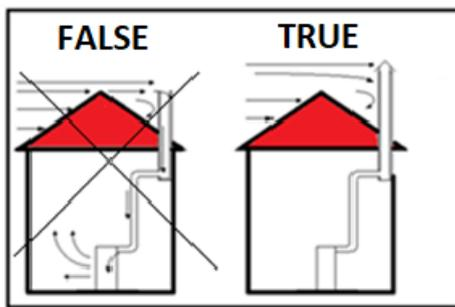
Chimney without flue cap and with flue cap
