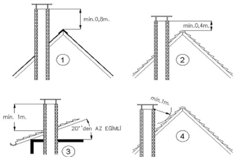
resistant to around 400°C. In order to obtain a better combustion and efficiency, all connections on the flue gas pipe must be sealed. The waste gas pipe should be connected to the chimney in the shortest way within the dimensions given in the diagram below. Horizontal connections and equipment such as elbows that reduce traction should be avoided.
