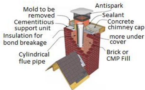
Smoke chimneys should not be placed on the outer wall of the building unless there is a technical necessity. The wall thickness of the chimney walls should not be less than the thickness of one brick. Perforated bricks and briquettes should never be used in chimney construction.
